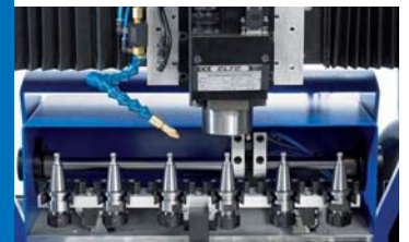
Spindle 2KW SK 20 with 6-times magazine
